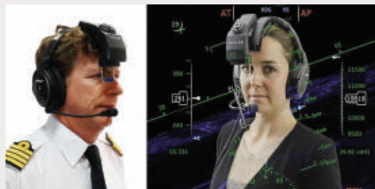
The TopMax commercial head-up display is based on military HUDs.
